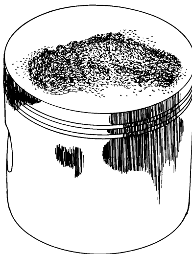
Damaged Piston Resulting from Detonation
